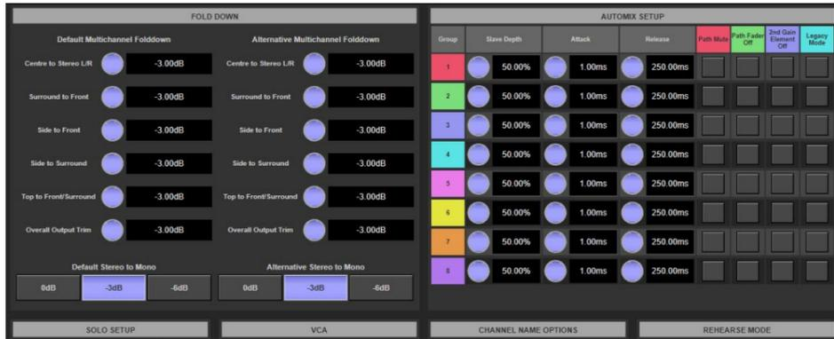
Main and alternate fold down coefficients are available, including controls for the side and top channels mean that standard 5.1, stereo and mono mixes include the precise amount of overhead or side contribution simply by routing the immersive channel or stem to a 5.1, stereo or mono bus. This greatly simplifies the process of simultaneously providing immersive and standard 2D program feeds.
