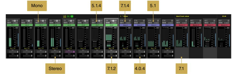
Channel View and S500 meterbridge path meters support all the path formats.
